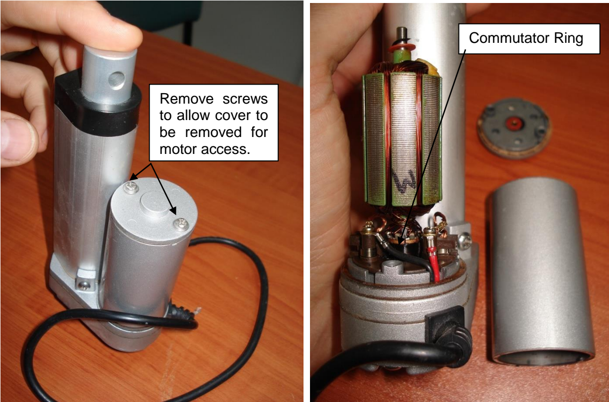
Figure 110 – Linear Actuator Disassembled (all J-Series)
