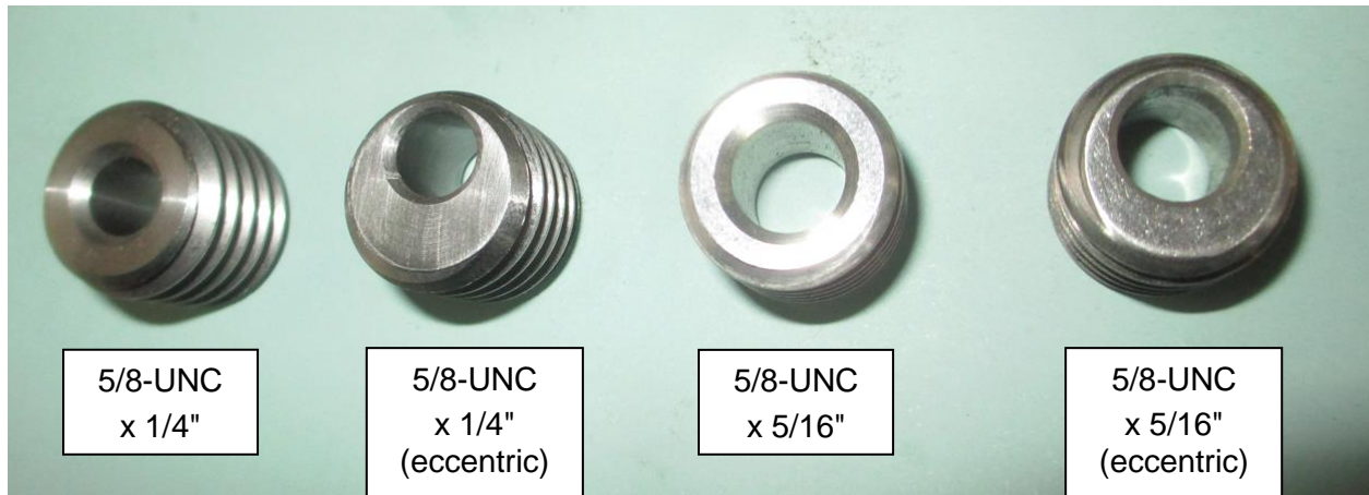
Figure 40 - stainless steel bushes used in Jabiru aircraft wing lugs
