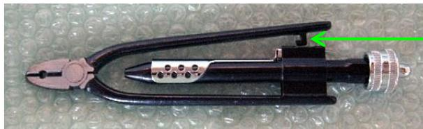
To use: lock the jaws onto both ends of your lockwire using the silver lock handle, then simply pull the "twist" handle at the back of the pliers and presto, perfect lockwire!
