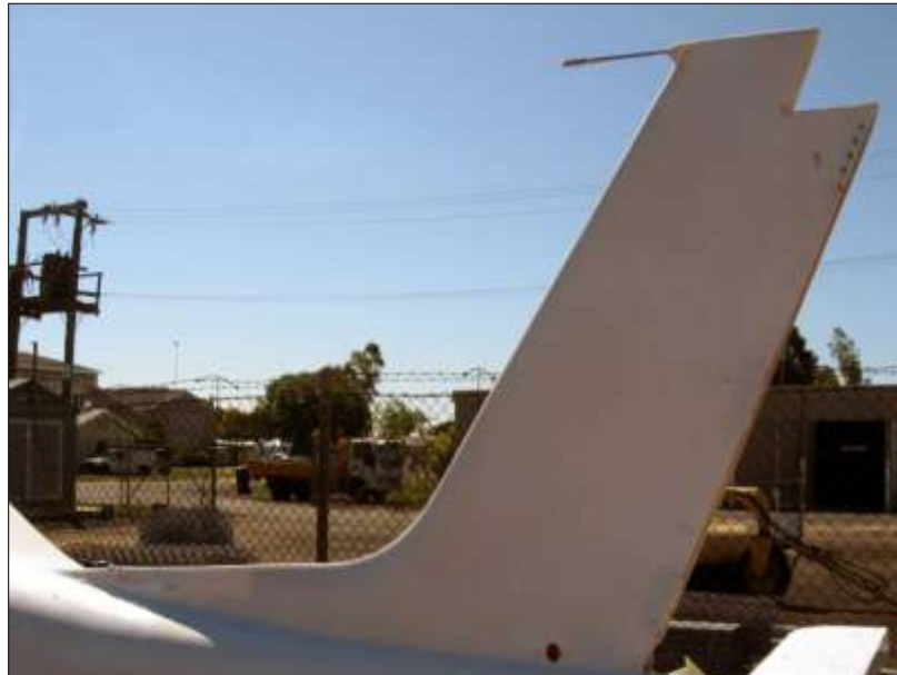
Completed vertical fin fitted to the fuselage
