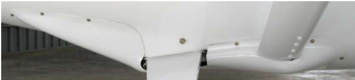
Right hand side strut/main gear fairing from below (top photo) and side on (above)
