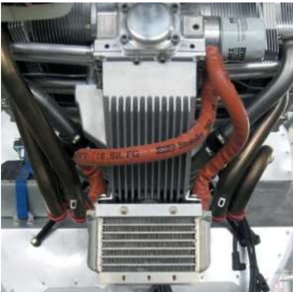
Completed oil line arrangement between the adaptor and the oil cooler
