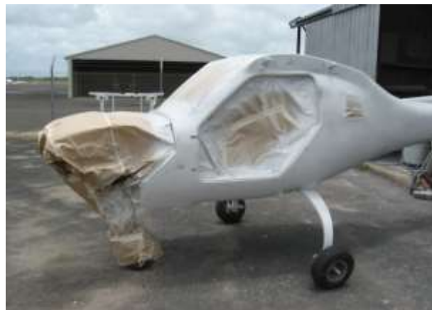
Masked and undercoated J170 fuselage
