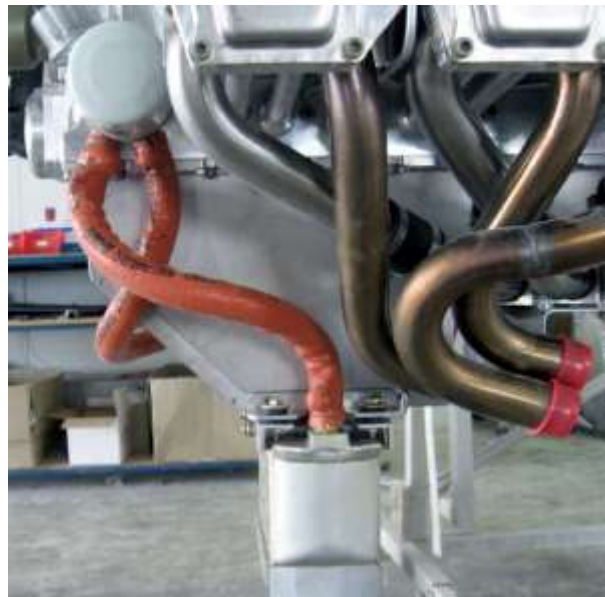
Completed oil line arrangement between the adaptor and the oil cooler
