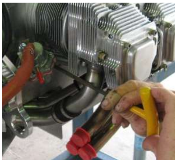
Remove the fuel pump from the engine
