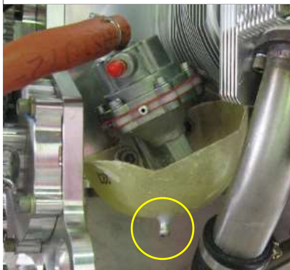
Re-fit the fuel pump with the drip tray underneath
