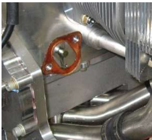
Clean the gasket and the spacer block
