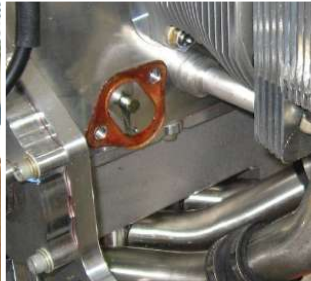
Clean the gasket and the spacer block
