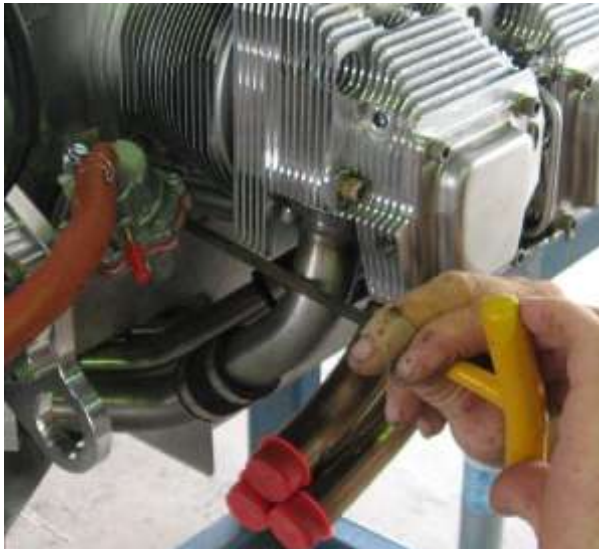
Remove the fuel pump from the engine
