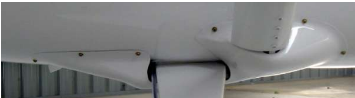
Right hand side strut/main gear fairing from below (top photo) and side on (above)
