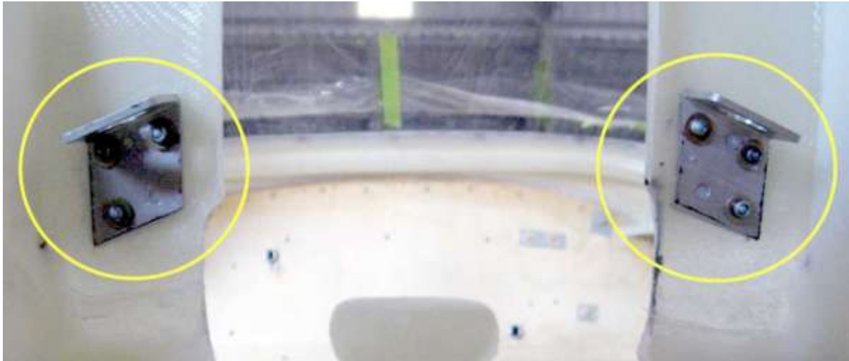
completed aileron cable mounts as viewed from the rear facing forwards
