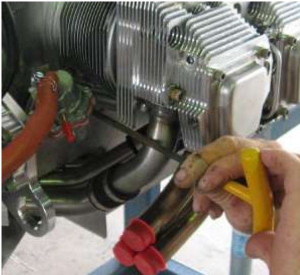
Remove the fuel pump from the engine
