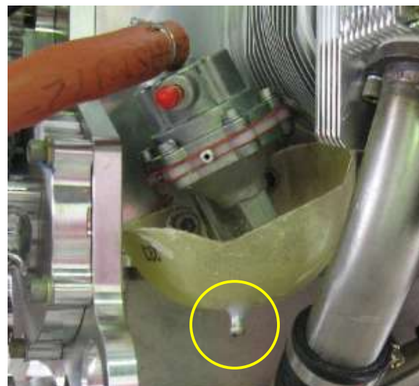
Re-fit the fuel pump with the drip tray underneath
