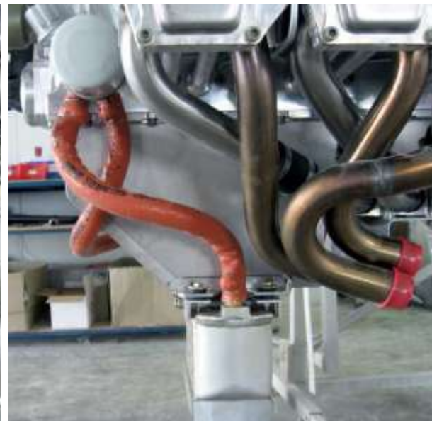
Completed oil line arrangement between the adaptor and the oil cooler
