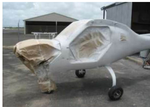
Masked and undercoated J170 fuselage
