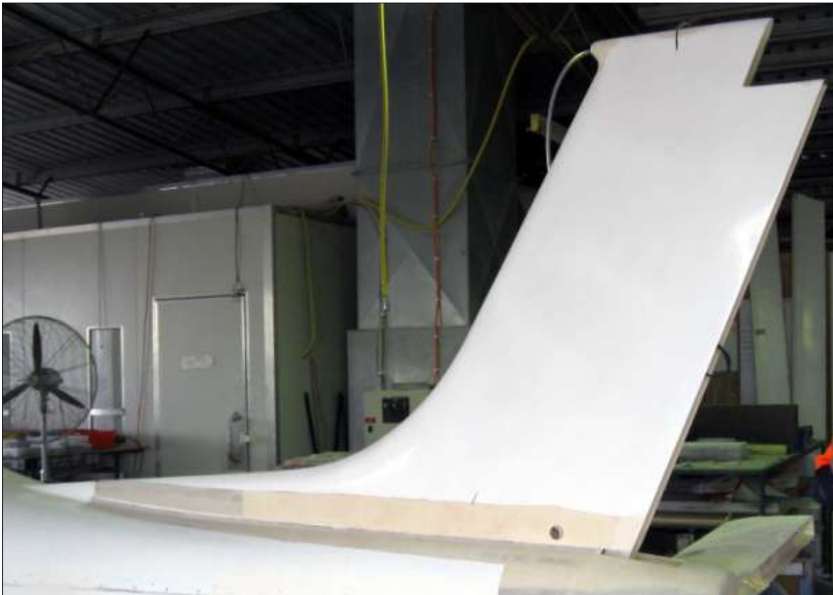
Vertical fin set in place with the peel cloth removed
