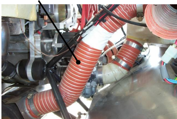
Figure 46. SCAT Hose Detail
