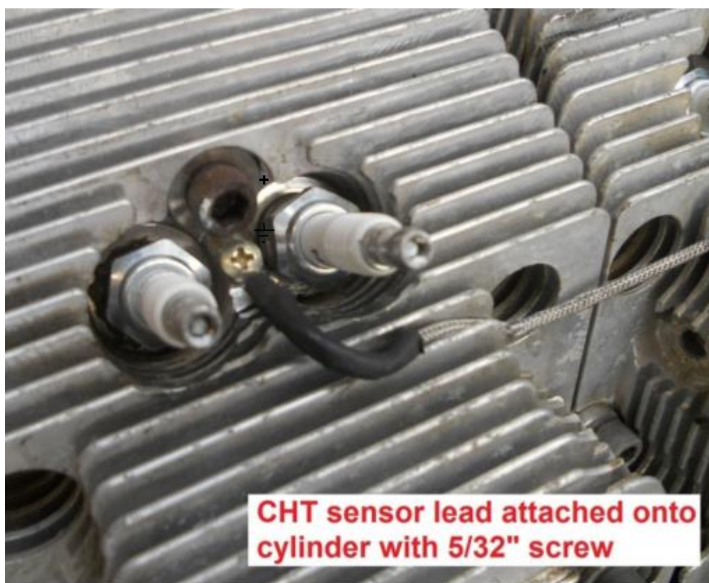
Figure 26. CHT sensor between plugs
