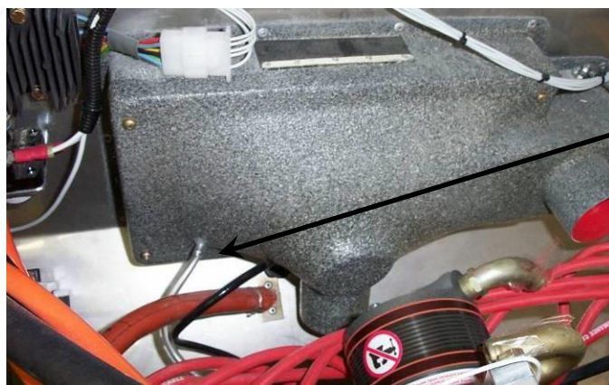
Figure 47. Balance Tube Detail
