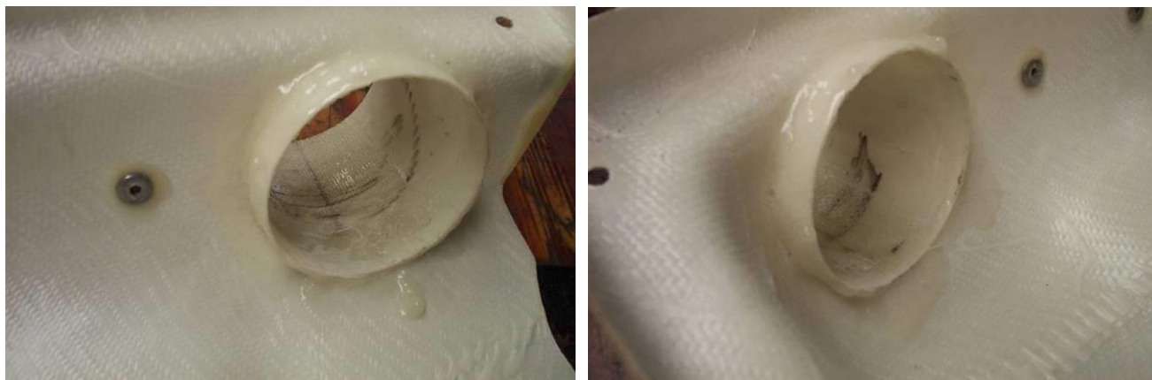
Figure 36. Air Filter Box Plumbing – Incorrect
