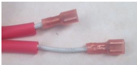
Figure 12 - Alternator leads must be of different lengths
