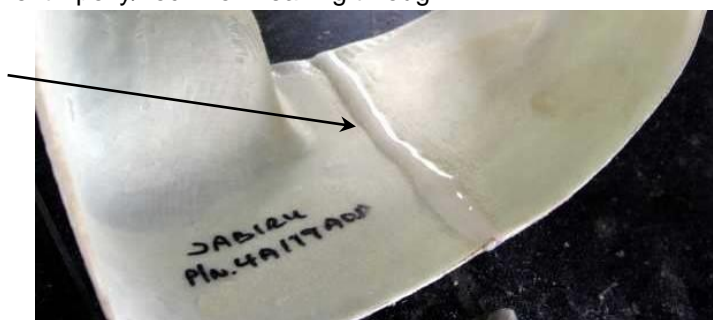
Figure 54. Ram Air Duct Front Seam
