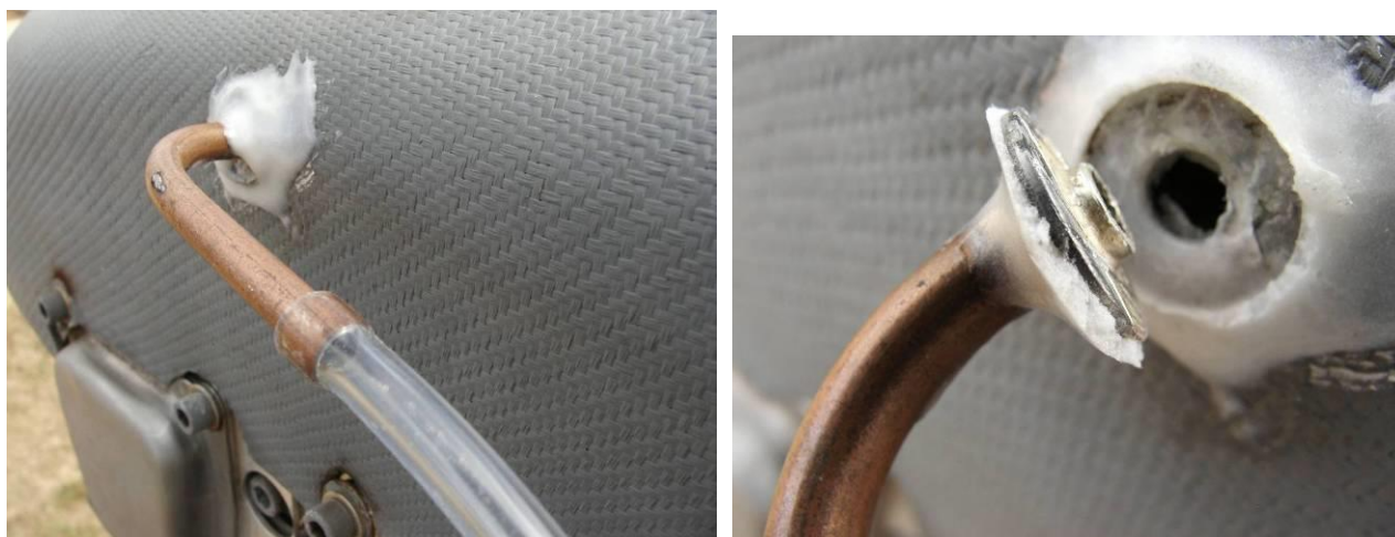
Figure 63: Ram Air duct pressure tapping.
