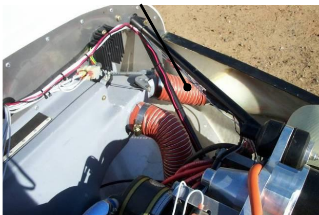
Figure 46. SCAT Hose Detail
