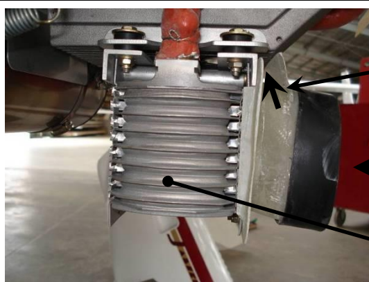
Figure 56. Oil Cooler Duct Design
