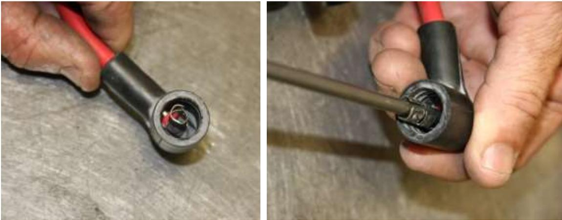
Figure 6 – Adjusting High Tension Lead Caps
