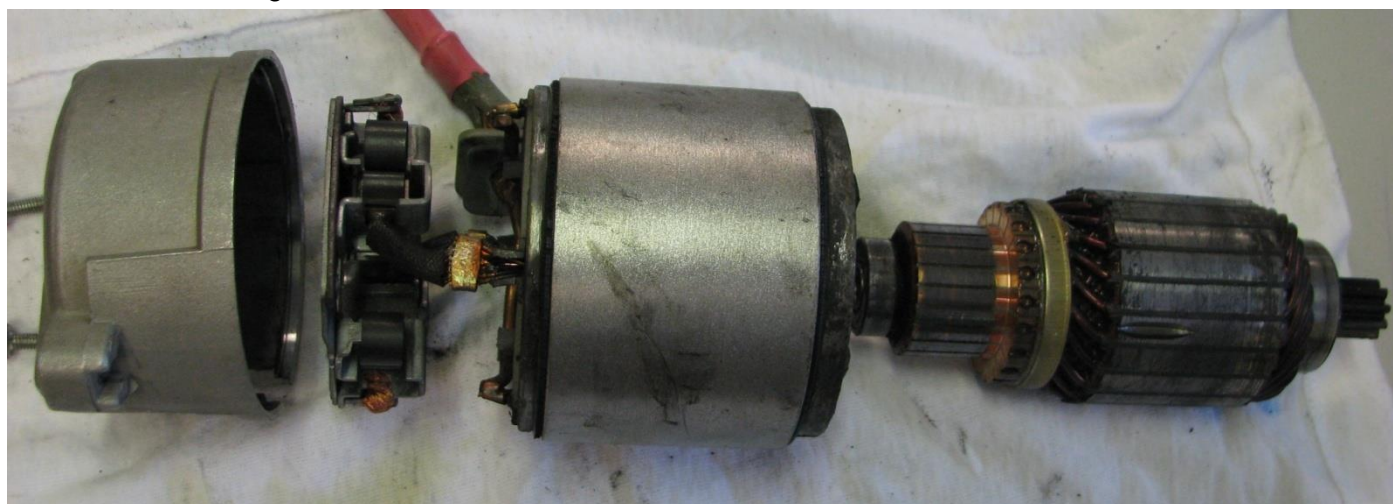
Figure 108 – Typical Disassembled Starter Motor
