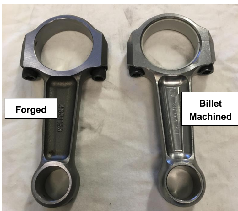
Figure 124 - Forged conrods vs Billet machined conrods
