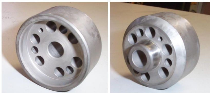
Figure 216 – Drilling Fixture – Crankshaft Side on Left, Flywheel Side On Right
