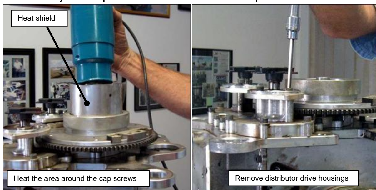
Figure 48 – Removing Flywheel Cap Screws & Distributor Drive Housings
