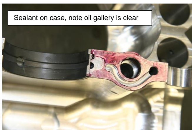
Figure 158 – Applying Sealant to Case, Fitting to Crank
