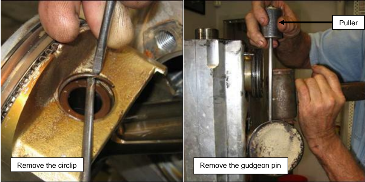
Figure 55 – Remove Pistons
