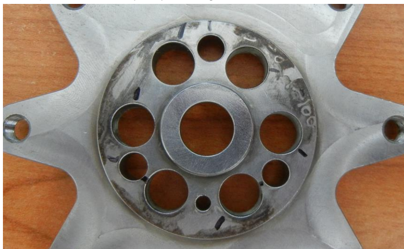
Figure 106 – Damaged Flywheel “Starfish”
