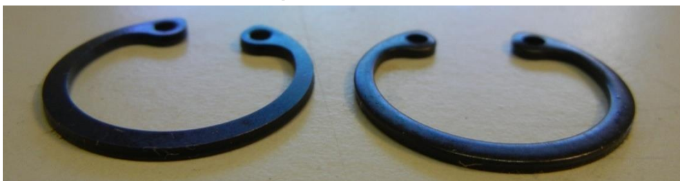
Figure 137 – The Two Sides of Circlips
