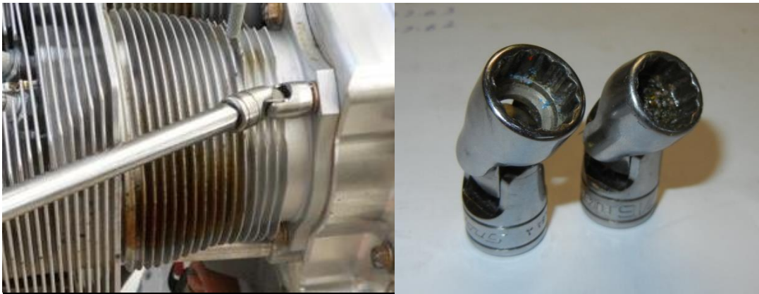
Figure 37 – Universal Joint tool FU14B
