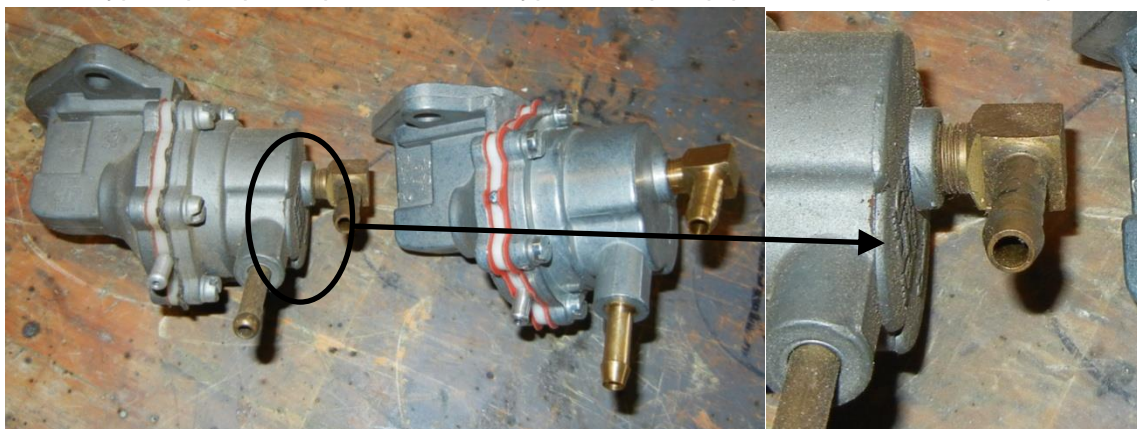
Figure 119 – Fuel Pumps (Type 1 on Left, Type 2 on Right)
