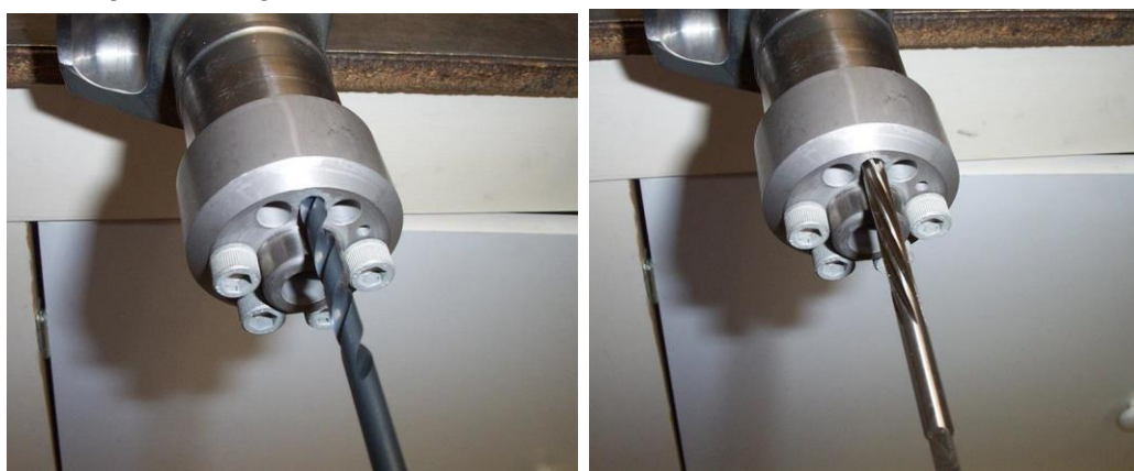
Figure 219 – Drilling & Reaming Crankshaft – ILLUSTRATION ONLY.
