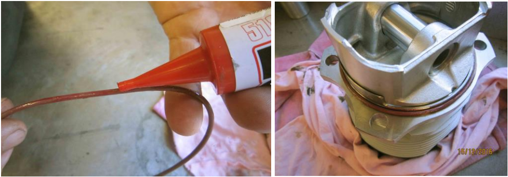
Figure 161 – Applying Sealant and O-Ring to Cylinder Base
