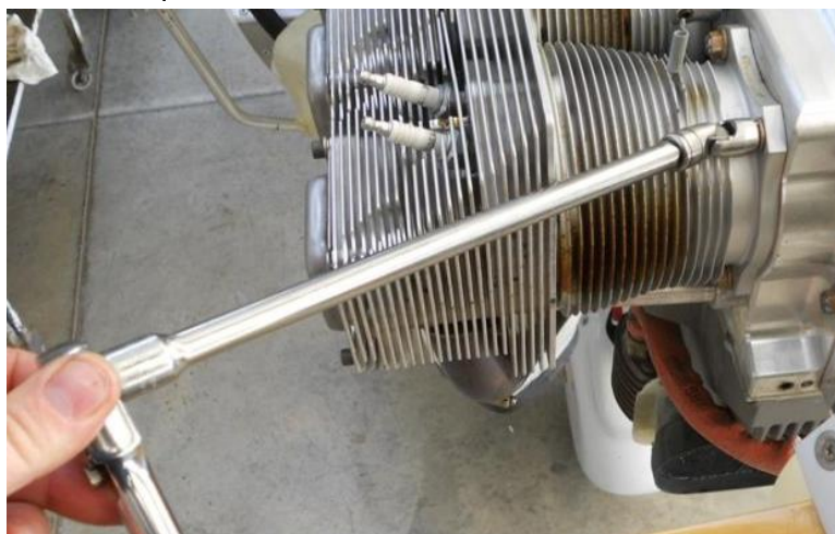
Figure 166 – Universal Joint tool FU14B (FU16B for 1/2" Socket)
