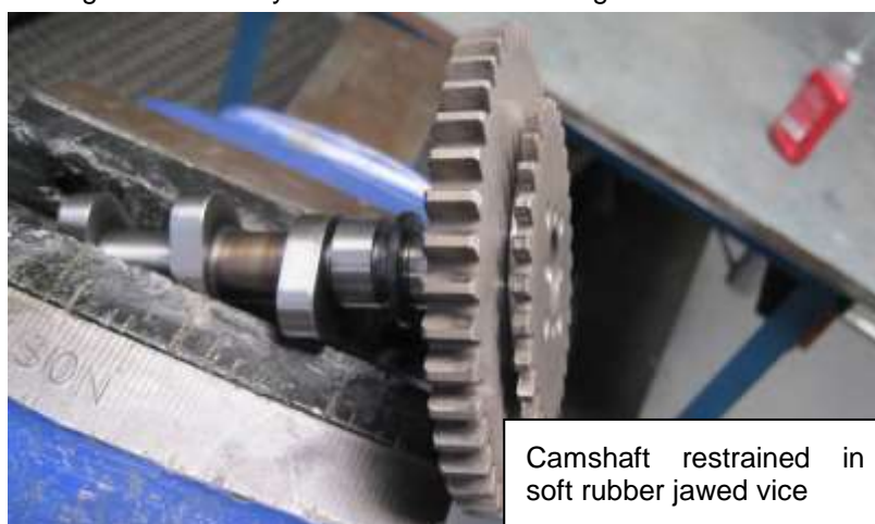
Figure 32 - Camshaft restrained in soft rubber jawed vice
