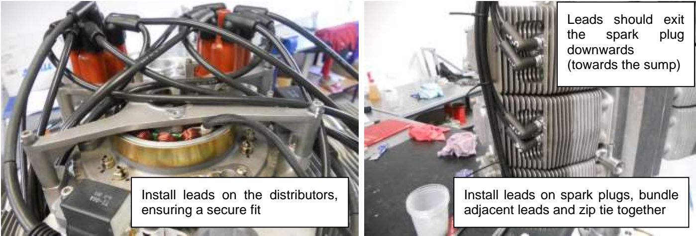
Figure 192 – Ignition lead installation
