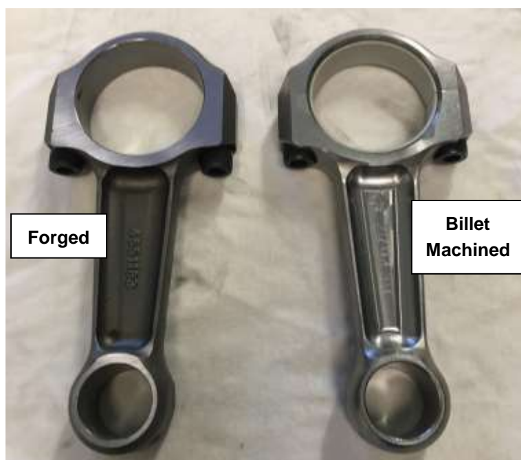
Figure 41 - Forged conrods vs Billet machined conrods
