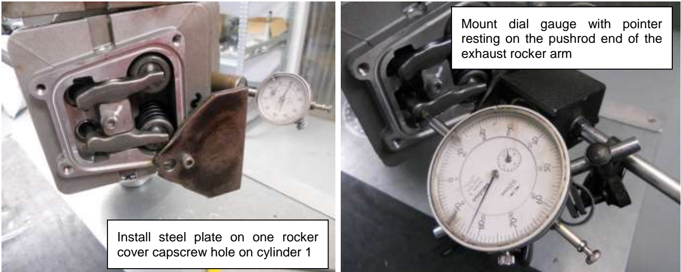
Figure 125 – setup dial gauge on number 1 exhaust rocker arm
