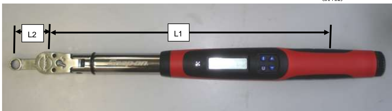
Figure 6 – Torque Wrench & Crows foot Adaptor Setting 1
