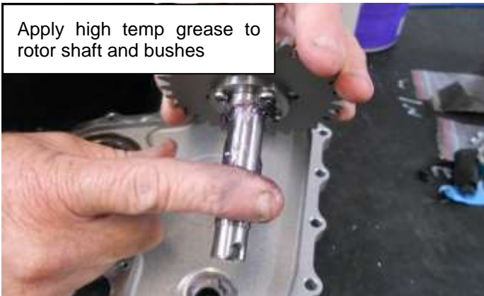
Figure 83 - Lubricating rotor shaft
