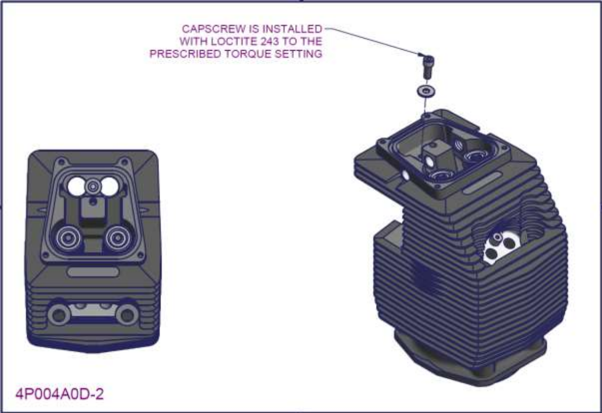
Figure 59 - 2200/3300 cylinder assembly 5a (external O-ring groove cylinder head)
