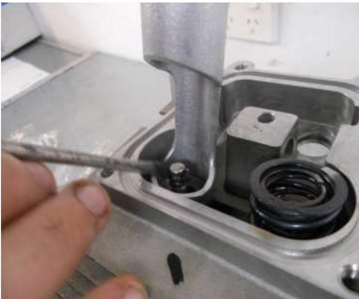
Figure 58 - Installing valve gear into the cylinder heads
