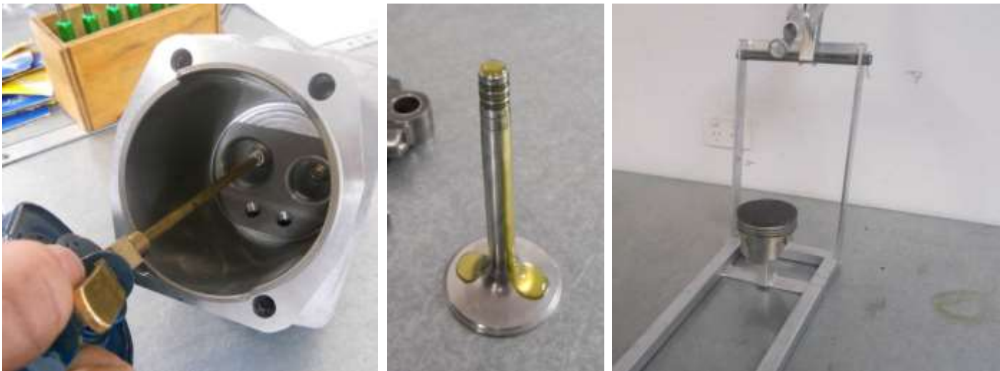
Figure 56 - Lubricating valves, seats and guides
