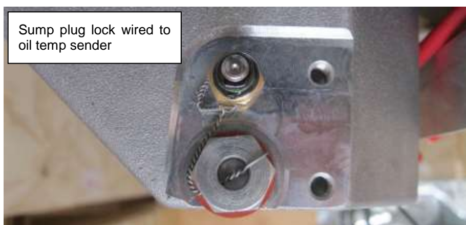
Figure 136 – Sump plug lock wiring
