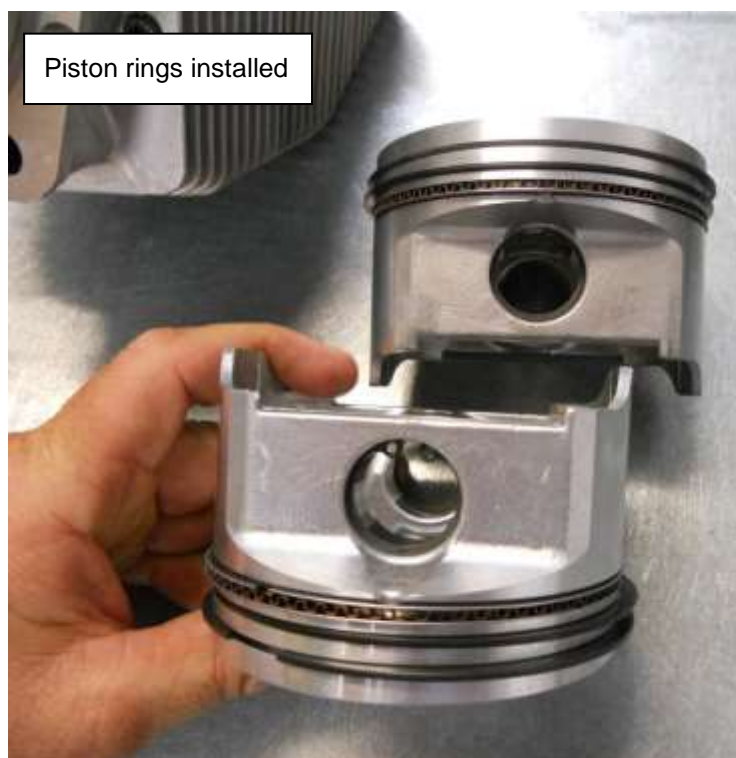
Figure 66 - Piston ring installation and oiling
