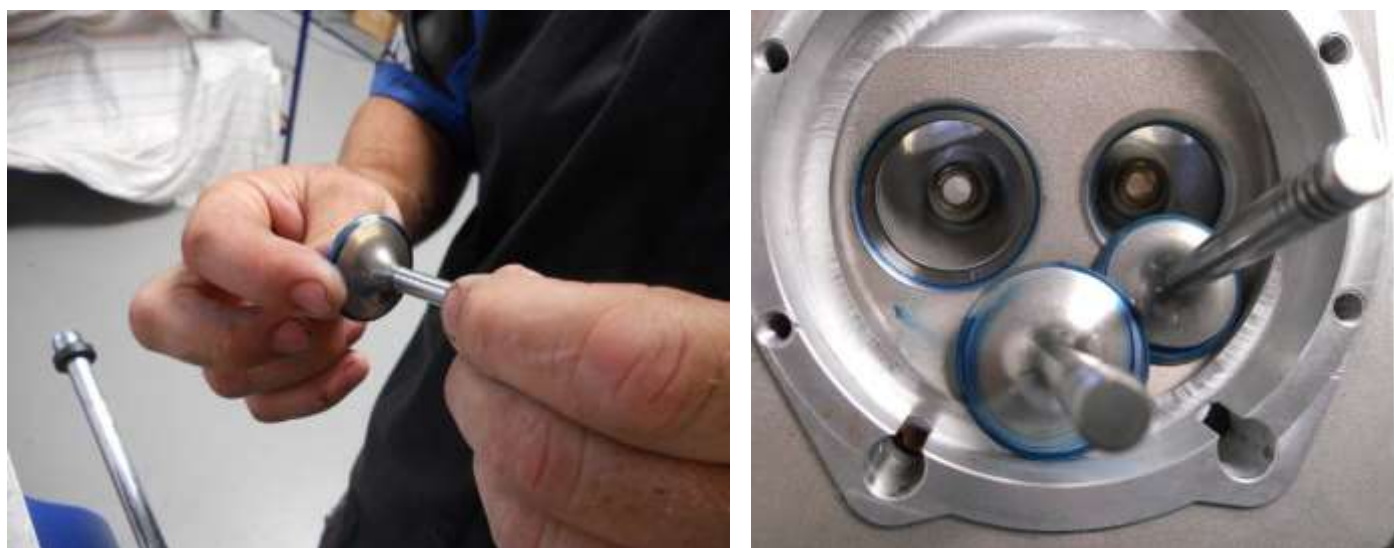
Figure 52 - checking valve sealing with bearing blue
