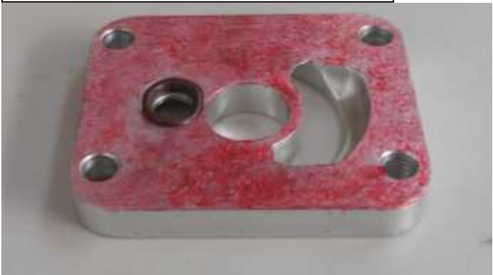
Apply Loctite 518 to the back plate (on the crankcase mating face only)
