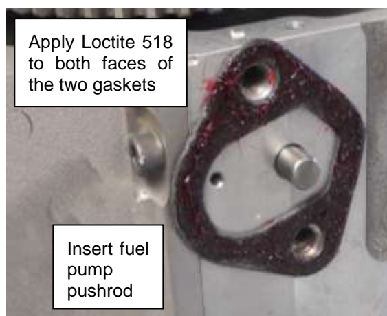
Figure 163 - Fuel pump installation
