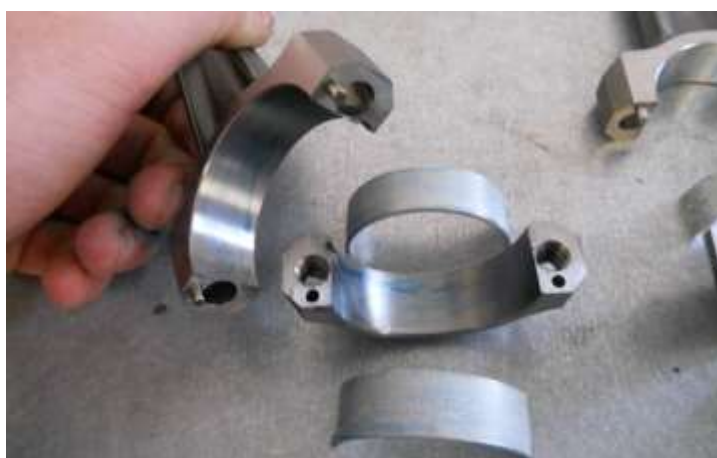
Figure 45 - Check for bearing blue transferal
