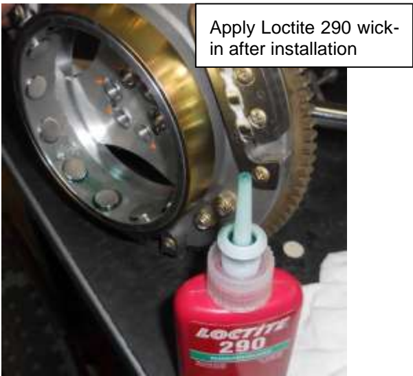
Figure 96 - Alternator magnet installation
