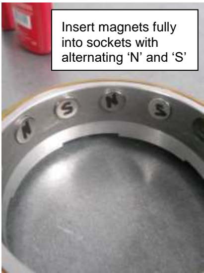
Figure 96 - Alternator magnet installation
