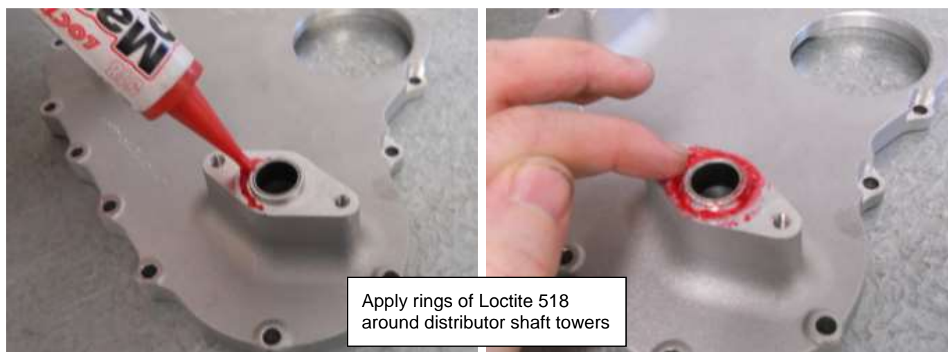
Figure 79 - Distributor mount plate installation
