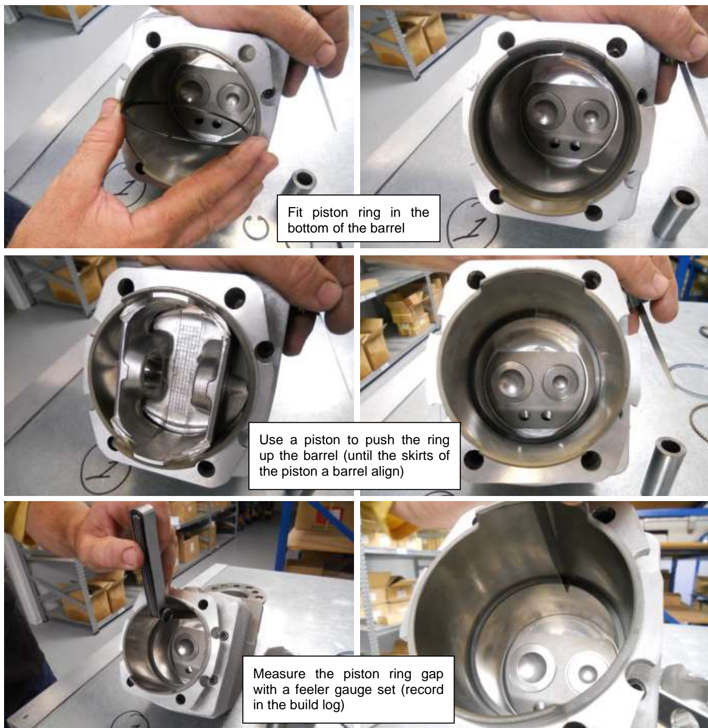
Figure 63 - Piston ring installation and measurement
