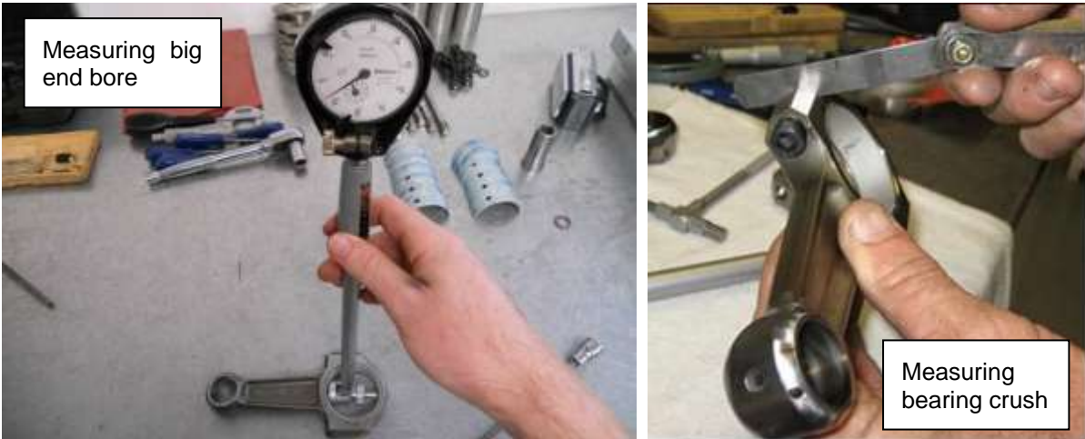
Figure 43 - Conrod measurements
