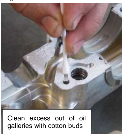
Figure 111 - Applying Three-bond to crankcase halves
