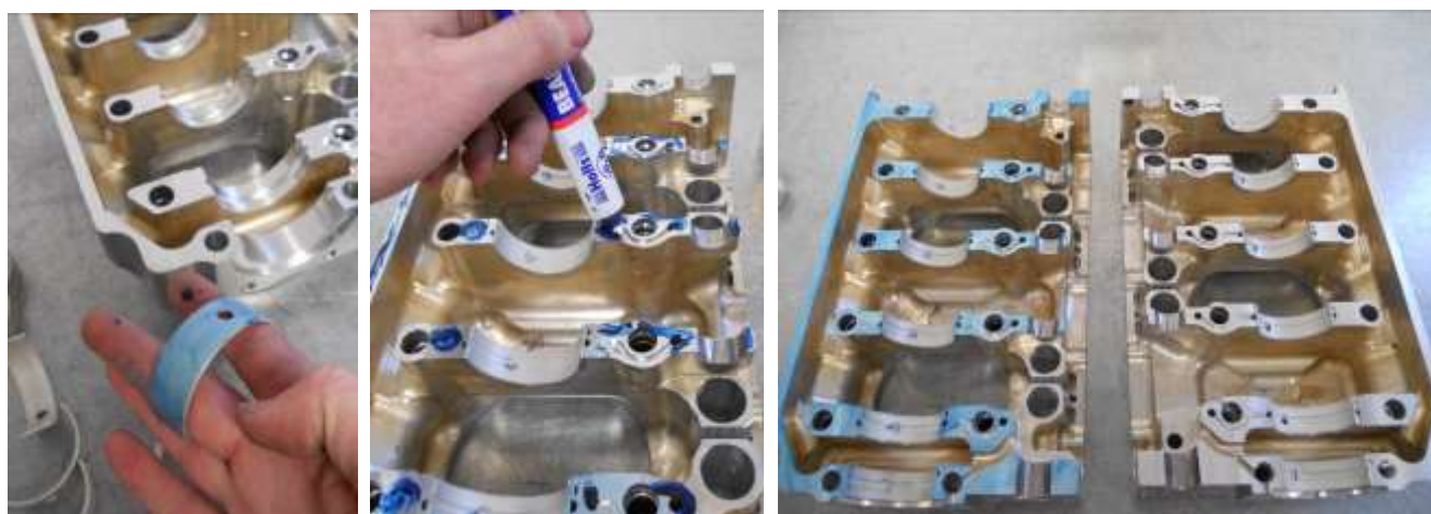
Figure 11 - Applying bearing blue to bearing shells and crankcase half
