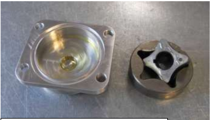
Lubricate housing and gears with engine oil
