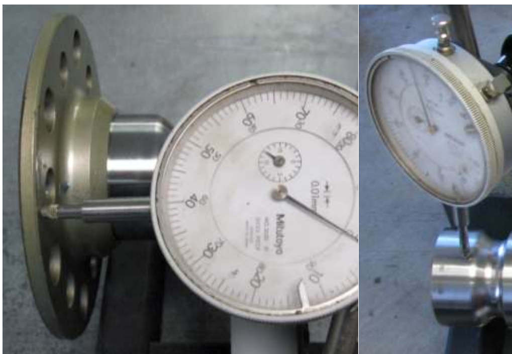
Figure 3 – Dial Indicator Position for Crankshaft & Prop Flange Run Out
