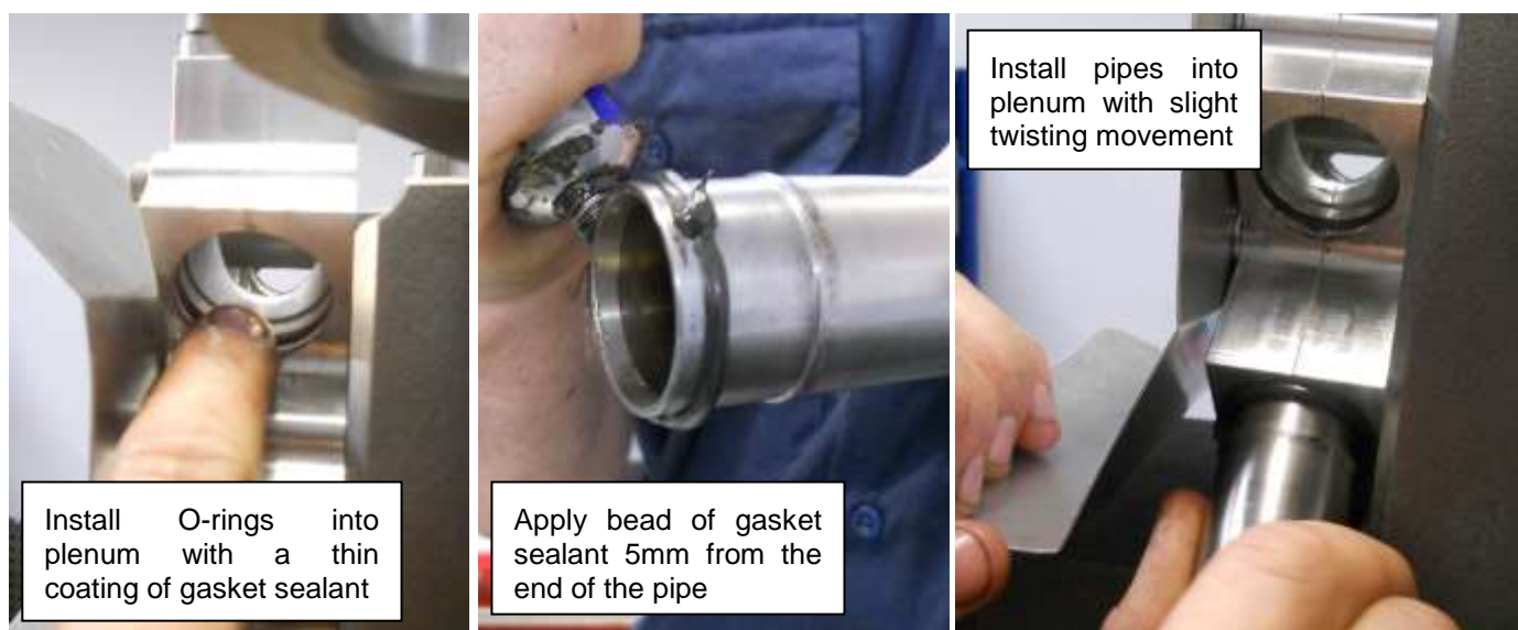
Figure 179 - Lower induction pipe installation
