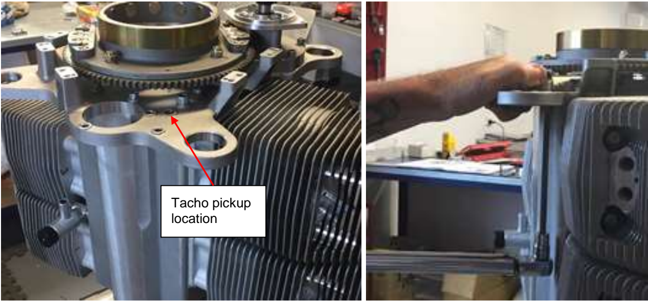
Figure 159 – Tachometer pickup installation
