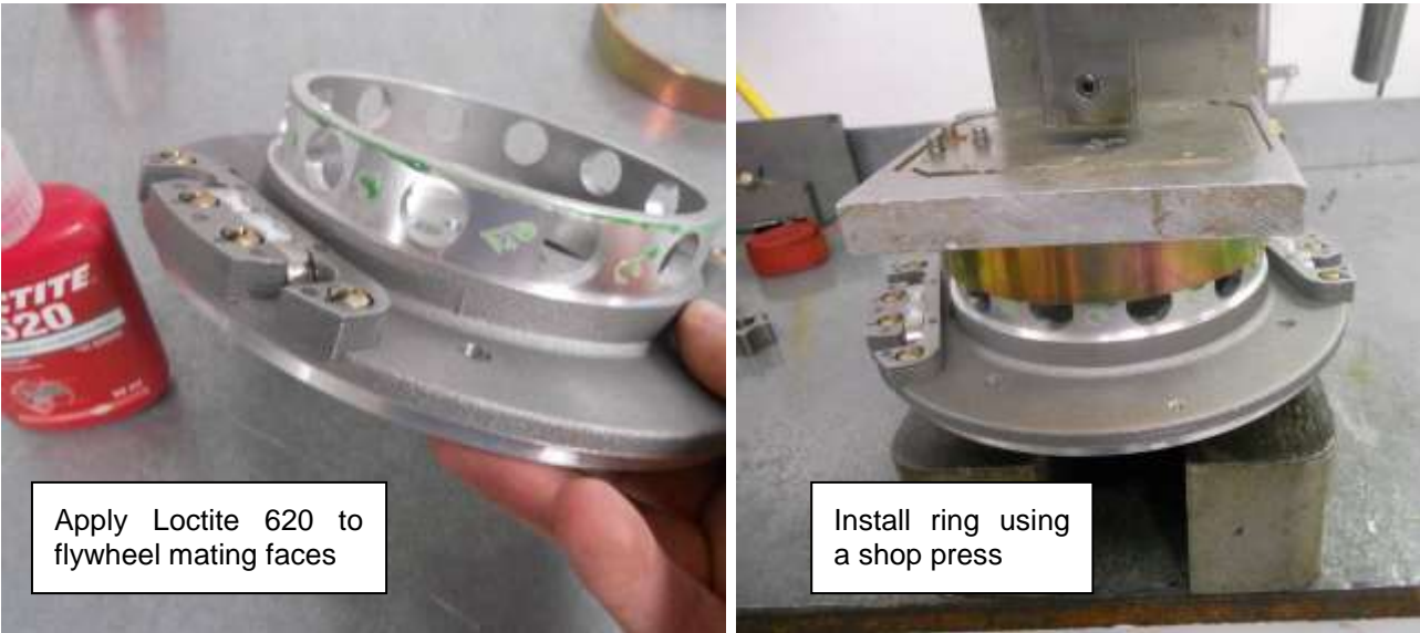
Figure 92 - Alternator magnet ring installation
