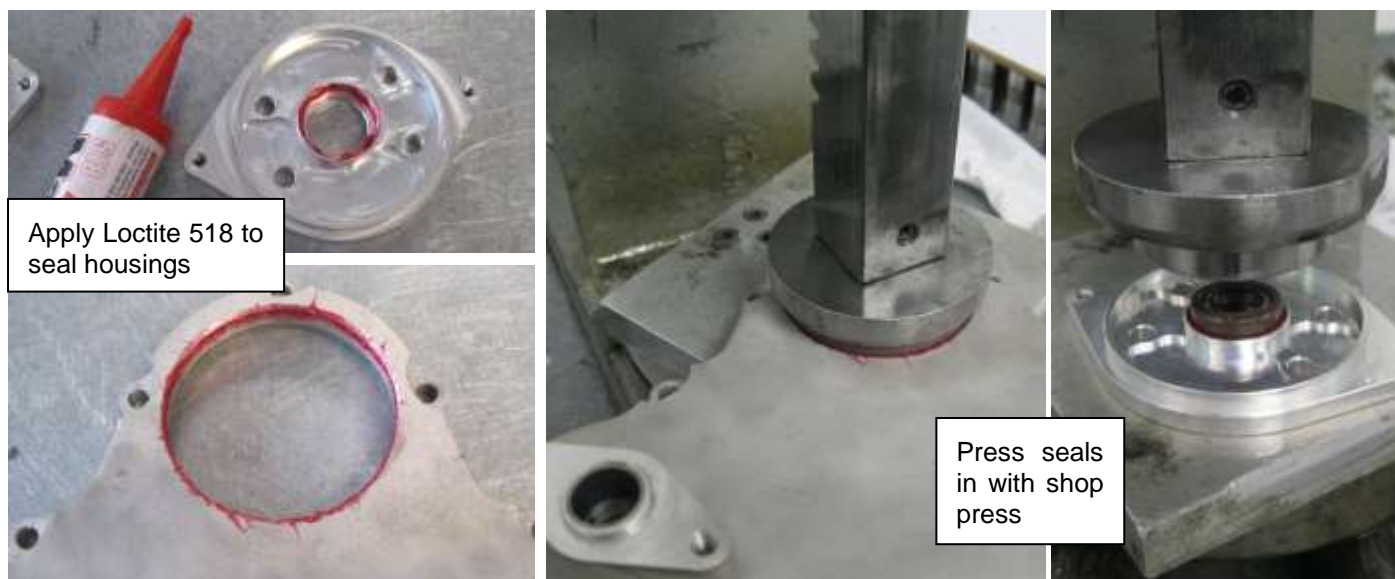
Figure 77 - Distributor gearbox seal installation
