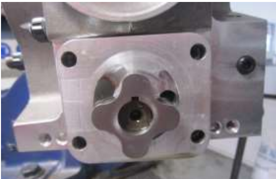
Align inner oil pump inner gear with woodruff key
