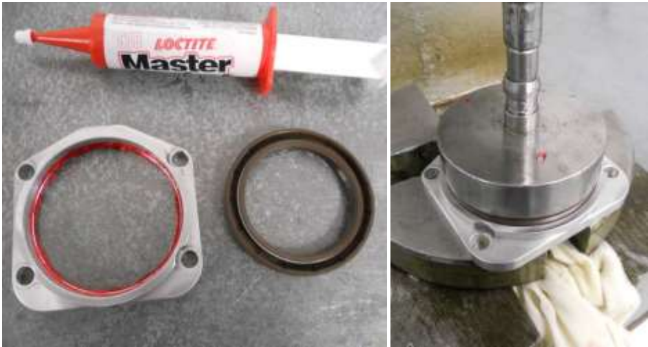
Figure 205 - External housing front seal installation
