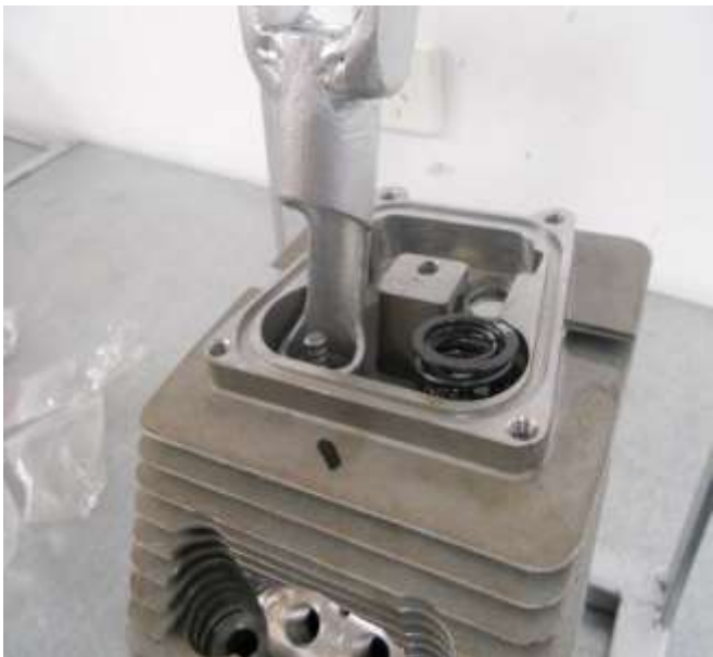
Figure 58 - Installing valve gear into the cylinder heads
