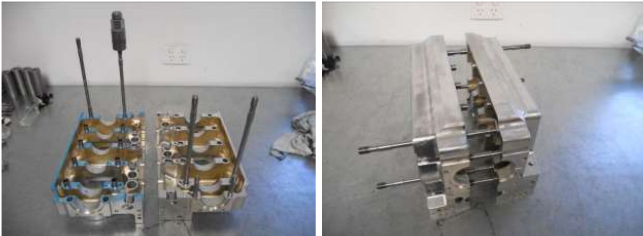
Figure 13 - Installing dowels and studs, pressing crankcase halves together
