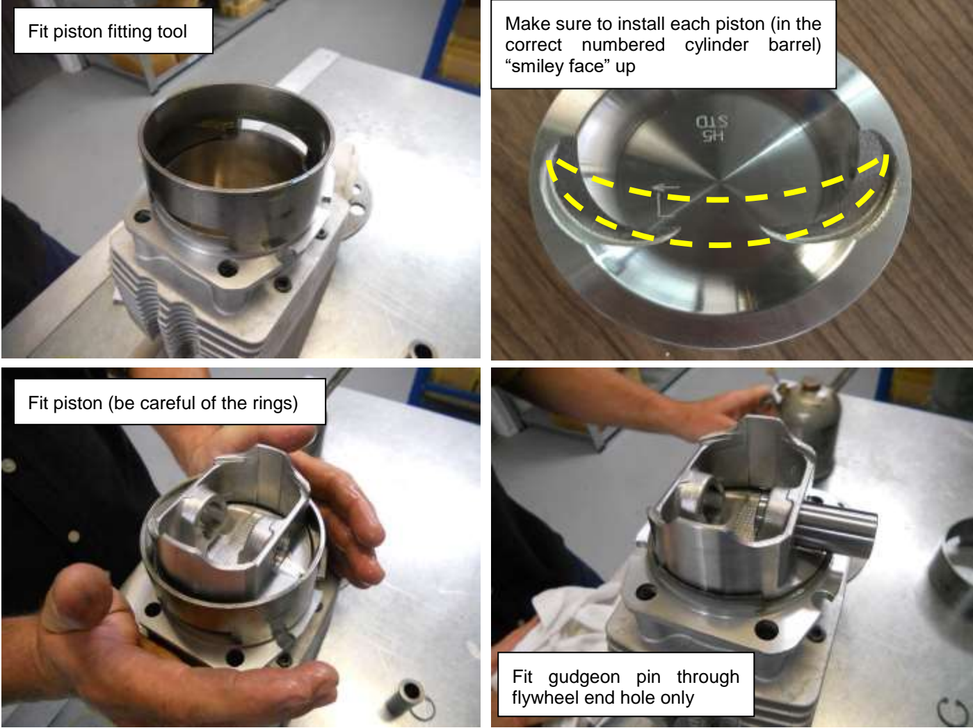
Figure 68 – Piston installation into the cylinder barrel
