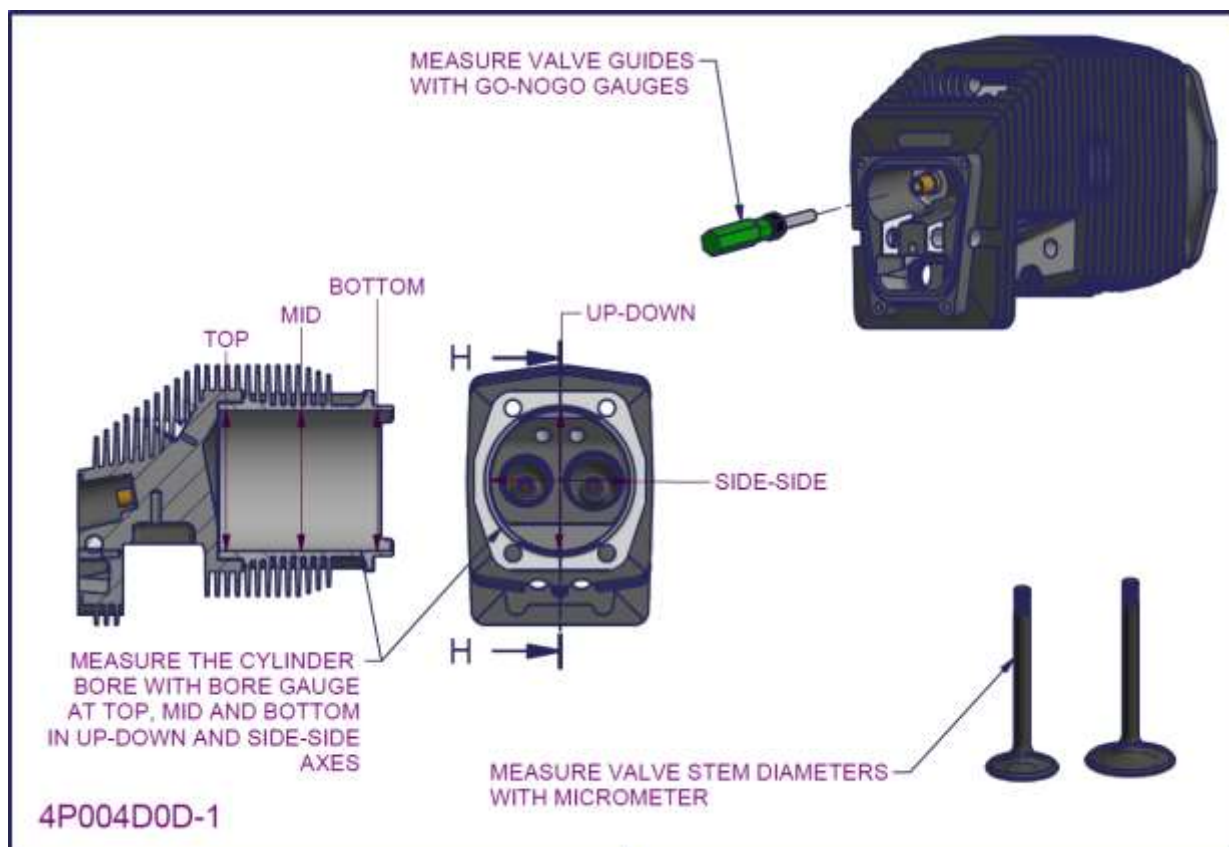
Figure 54 – 2200/3300 cylinder assembly 2
