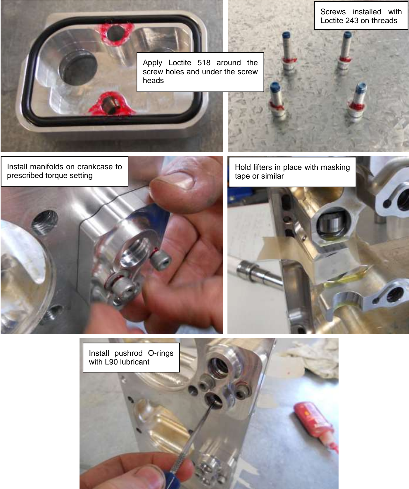
Figure 25 - pushrod manifold installation
