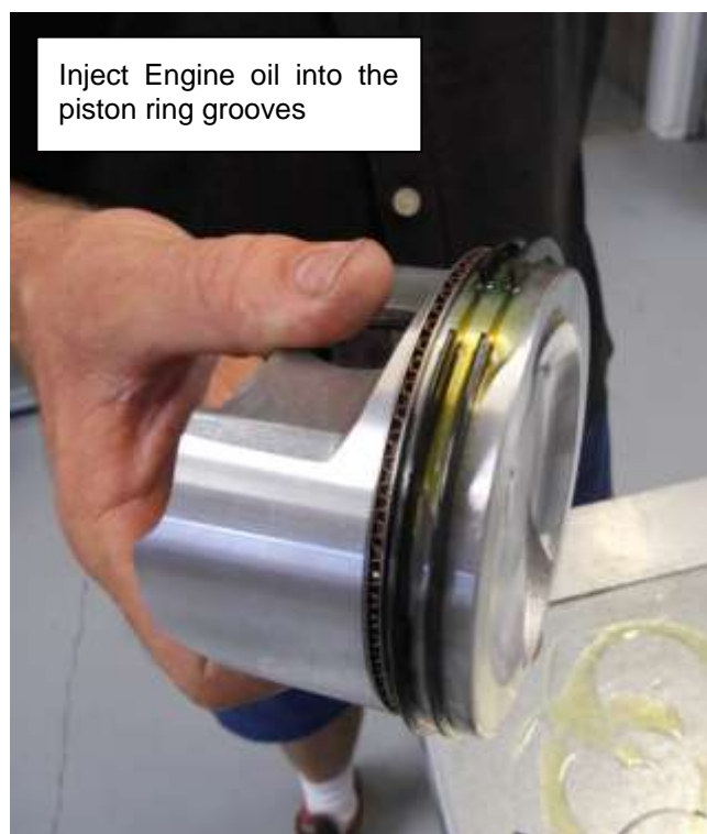
Figure 66 - Piston ring installation and oiling
