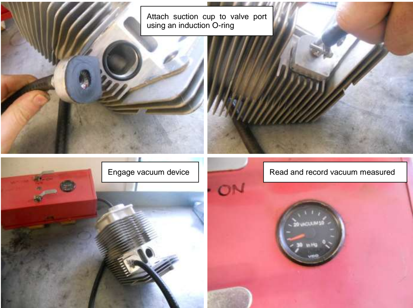
Figure 53 - Using a vacuum check to assess the valve sealing quality
