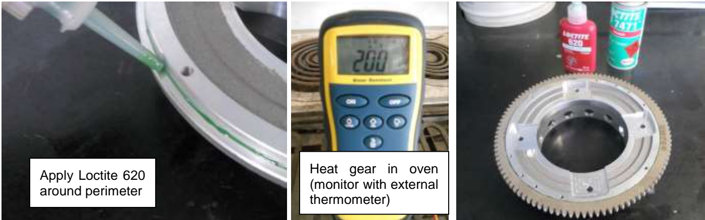
Figure 94 - Starter ring gear installation
