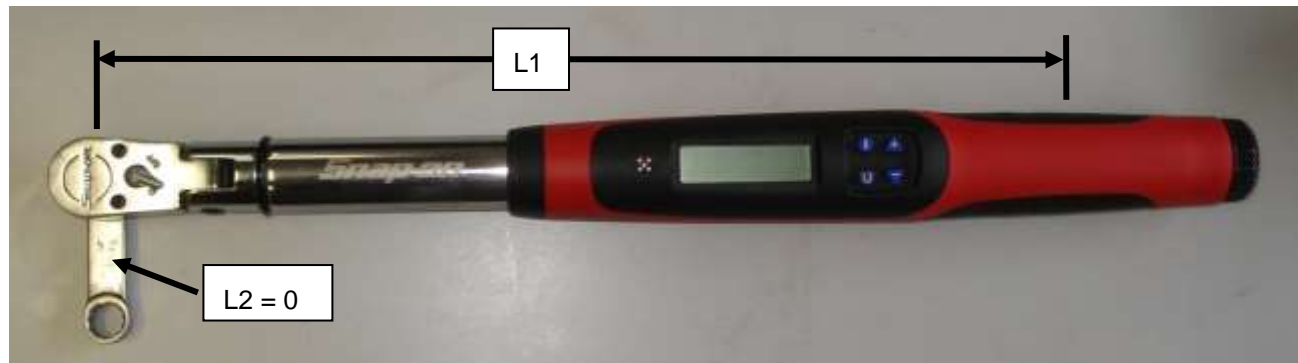
Figure 7 – Torque Wrench & Crows foot Adaptor Setting 2
