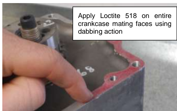
Figure 148 - Applying Loctite 518 to crankcase faces
