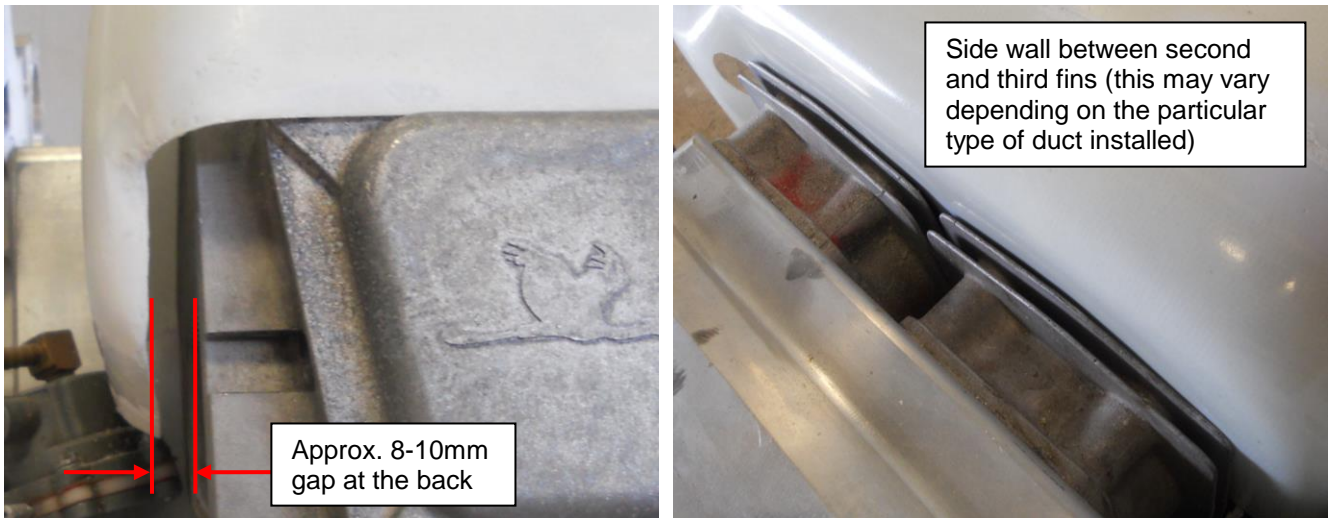
Figure 44 - Position ram-air duct on engine
