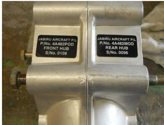
Figure 4 - Propeller hub indexing arrows
