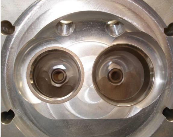
Figure 3 – Early “High Octane” Combustion Chamber
