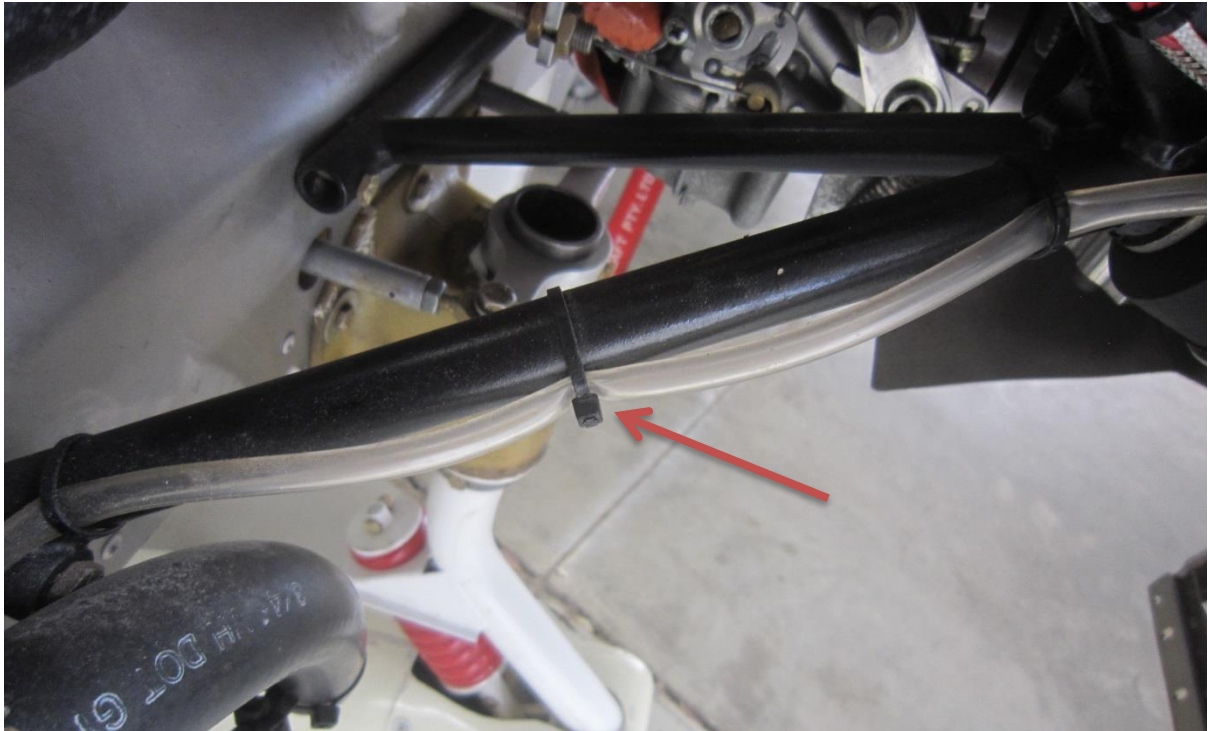
Figure 1: Crushed drain line.
