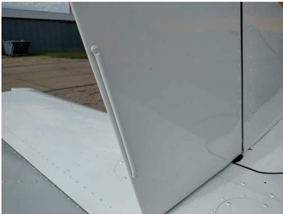
Permanent bump trim using 1/4" Aluminum tubing.
