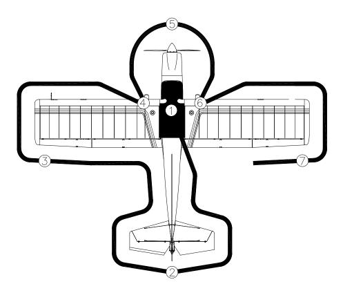
FIGURE 10-08. Preflight Inspection Sequence
