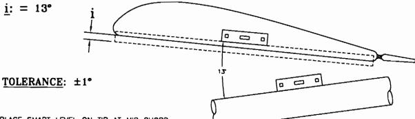
PLACE SMART LEVEL ON TIP AT MID CHORD AND ZERO. PLACE ON BOOM TO READ DEGREE OF INCIDENCE RELATIVE TO BOOM. FOLLOW THIS PROCEDURE FOR THE TAIL INCIDENCE AS WELL.
