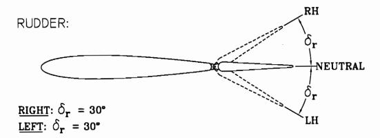
CHECK FOR CONTACT AGAINST ELEVATOR. ADJUST TO AVOID CONTACT
