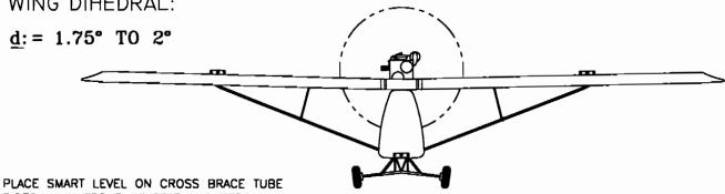
DIRECTLY IN FRONT OF SEAT AND ZERO. PLACE ON WING CENTERED BETWEEN RIBS AT STRUTS.
